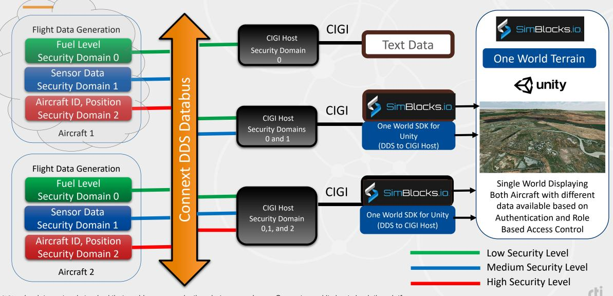
CIGI: wire data protocol standard that enables communications between an Image Generator and its host simulation platform
